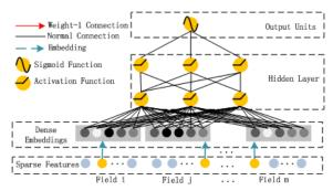
Figure 3: The architecture of DNN.
