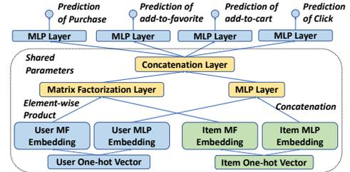
**Figure 6: Multi-Task recommendation network in the evaluation. The shared bottom layers is the combination of MLP layer and matrix factorization layer, which is widely adopted for recsys in both academia [10] and industry [6, 25]**
